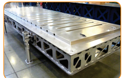
High-tolerance Invar Production Tooling
