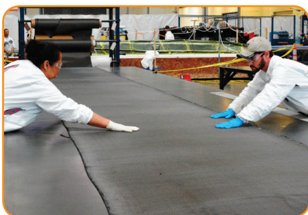
Carbon Fiber Lay-up
