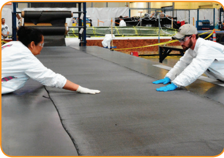
Carbon Fiber Lay-up
