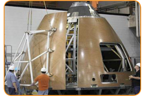
Large, one-off, composite skins for Orion
