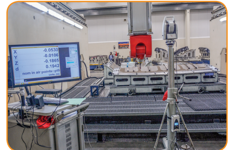
Laser Metrology machine alignment ensures high tolerance results
