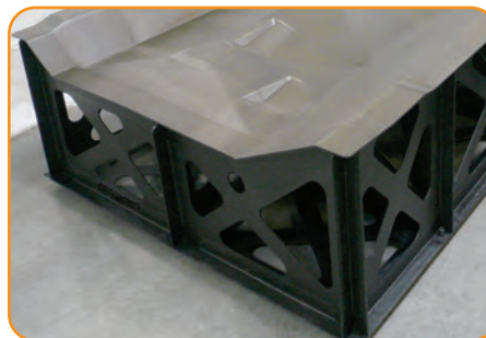
Carbon/Epoxy Panel Eggrate
