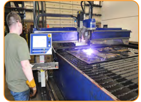
Messer Titan III Plasma Cutter 10ft x 20ft Bed x 2in Thick
