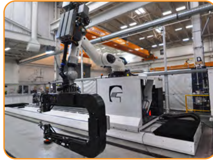
Genesis Non-destructive Testing (NDT) 115 Equipment Robotic Inspection Workcell
